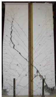
Flexure-diagonal tension (Tran, 2012)
