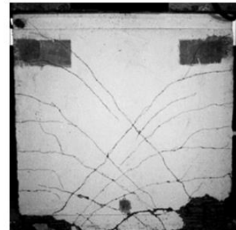
Flexure-shear-sliding (Salonikios et al., 1999)
