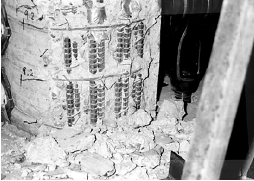
Figure E2-10 Specimen C-1 from Saadatmanesh et al. (1997) following failure, shown as an example of a column with bond failure as its primary damage state.
